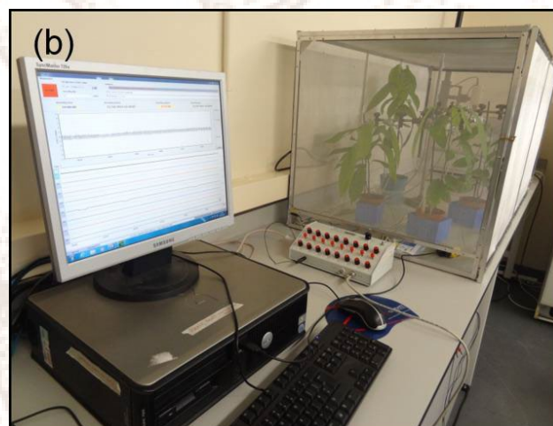
A multi-channel EPG arrangement allowing for the monitoring of up to eight separate mealybug/cacao feeding combinations simultaneously
