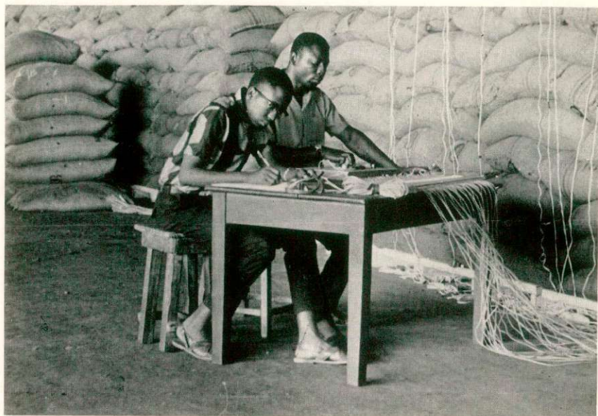
Measuring temperatures with thermistors inside a stack of cocoa beans at Apapa.
