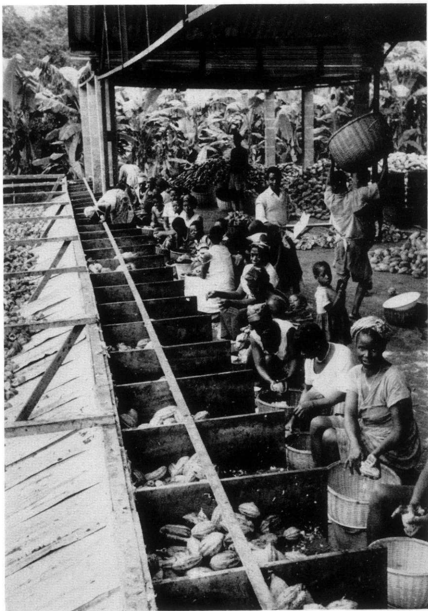
The pod – opening scene. The husk hoppers on the left are emptied direct into trailers.
