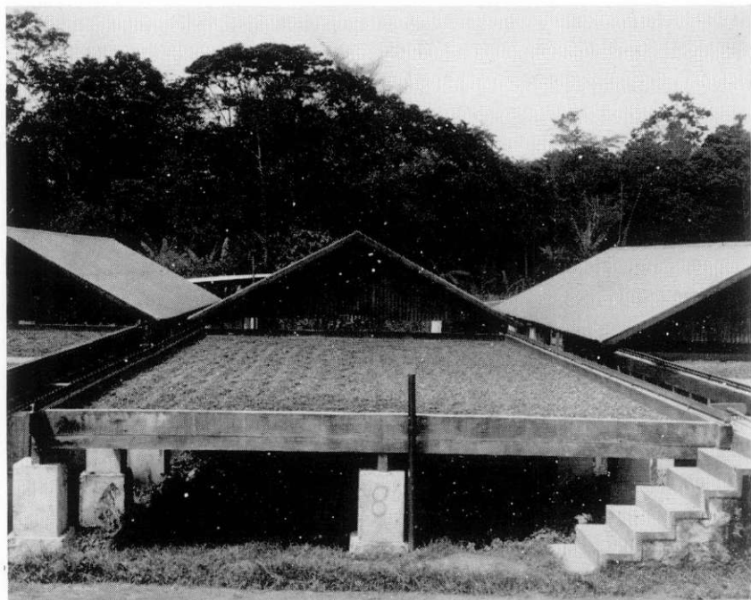
Beans drying on a barcaca—sliding roof dryer.
