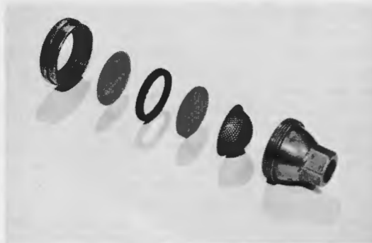
Fig. 3. Hollow cone or swirl nozzle—(left to right) cap, orifice plate, spacing washer, swirl plate, strainer and body.
