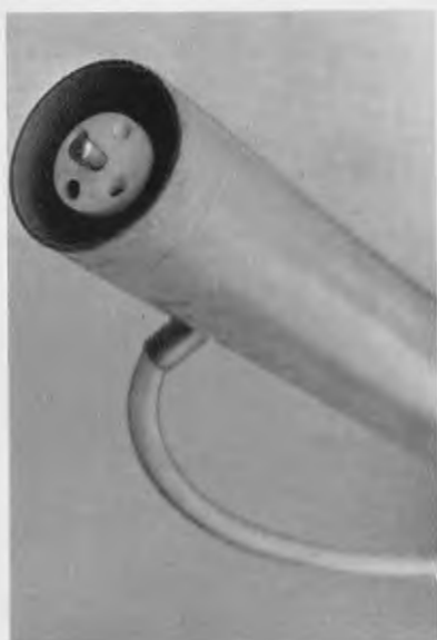
Fig. 6. Rotating disc nozzle in air discharge tube.
