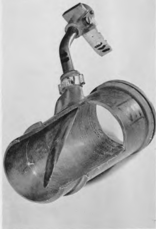
Fig. 7. Air-blast nozzle showing metering jet.
