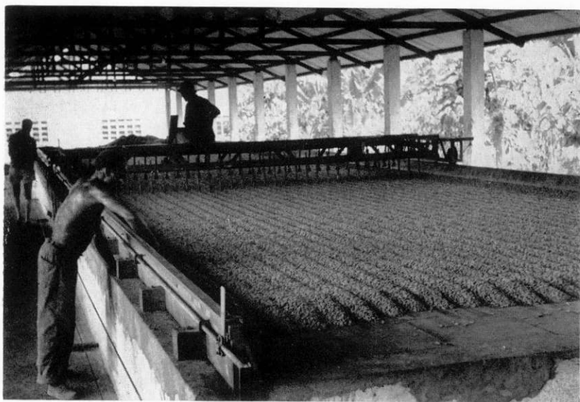
Slate drying floor with mechanical rake.
