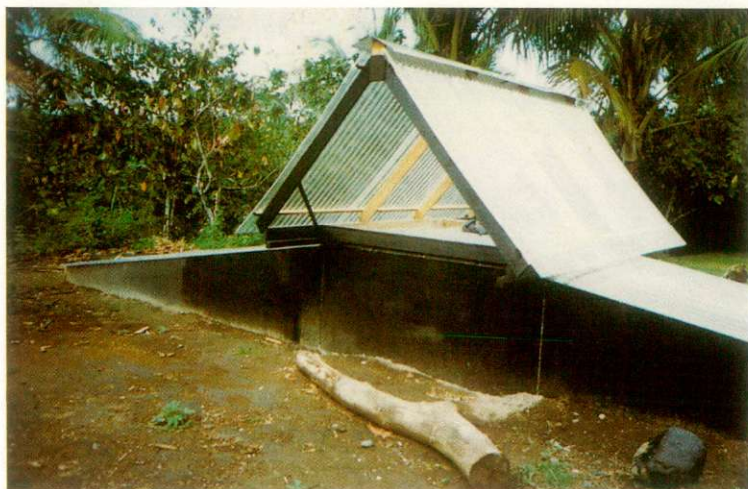
PLATE 1: SOLAR DRIER WITH ROCKS PAINTED BLACK AS SOLAR COLLECTORS AND COLLECTOR COVERS AND ROOF OF CLEAR POLYCARBONATE
