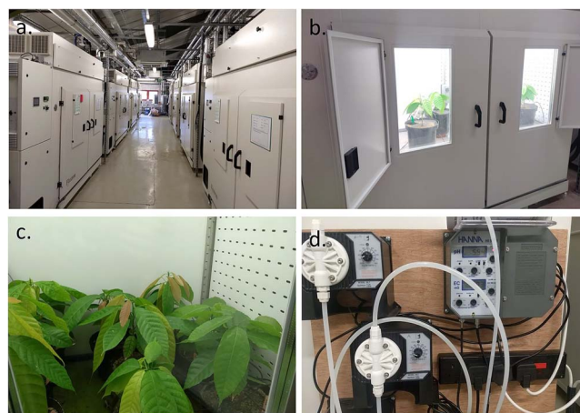
Figure 1. Growth cabinets used for the experiment (a and b), juvenile cacao plants (c) and fertigation control (d).
